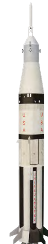
1965–1975 Saturn 1B rockets were mostly used to bring Apollo ships into low Earth orbit.
